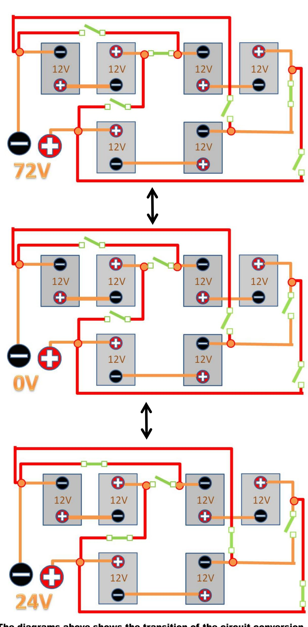
**Circuit Conversion from 72V to 24V**
