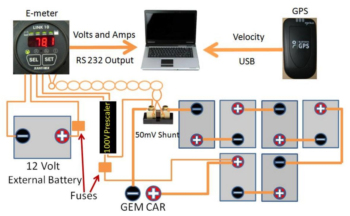
The block diagram above shows how the e-meter was The laptop recorded all the data from the e-meter and GPS using matlab. **E-meter measures:**
