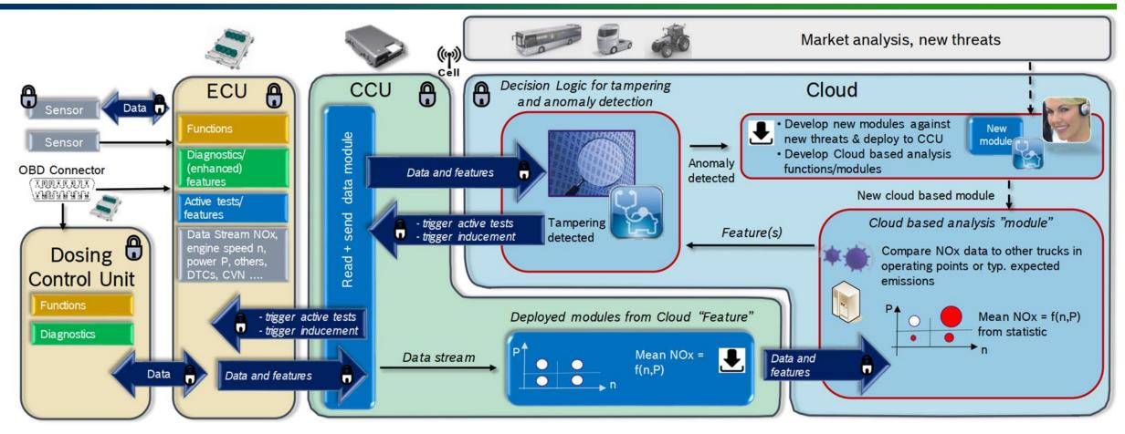
Our concept: combining the cloud capabilities with the engine management system and after-treatment controls and sensors
