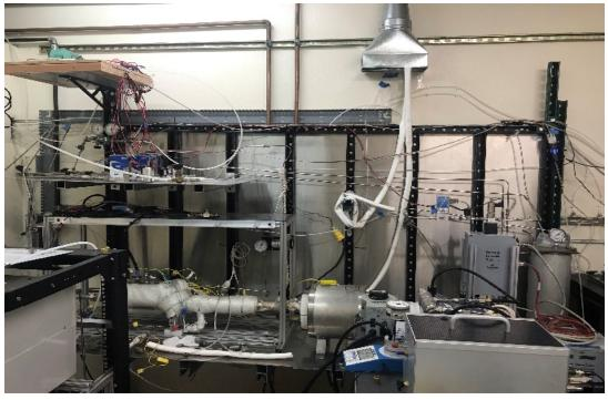
High flow bench to simulate exhaust conditions while calibrating and comparing with an FTIR and PM (miniCAST)
