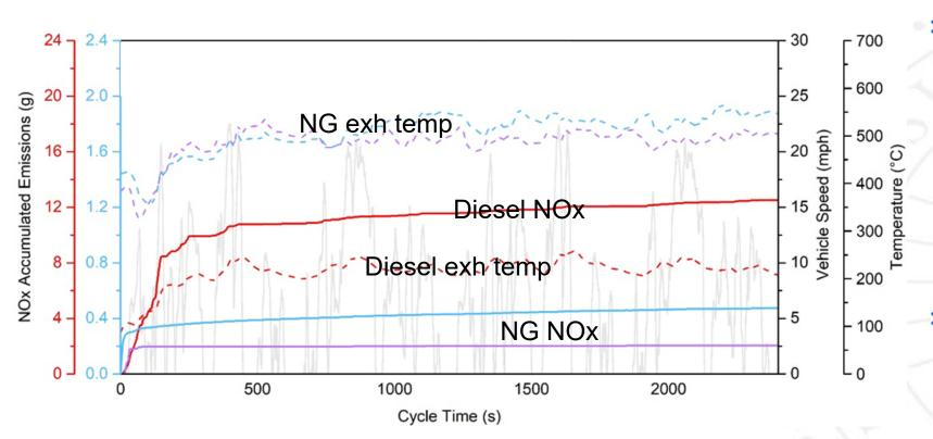
If the test cycle were 4 hrs long (typical for a fleet), the emissions for the NG vehicle would **decreased** by a **factor of 6** where for the diesel it would only reduce by a factor of 2
