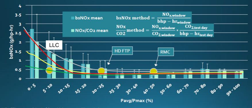
HHD with NOx FEL ≤ 0.20 g/bhp-hr | 85 vehicles, 2.90 million windows Work-windows are calculated over continuous seconds. Consecutive windows have overlapping seconds. Error bars are SD of the mean.
