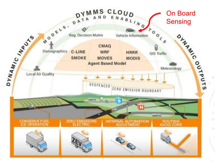
• The Dynamic Mobility Management System will collect data from vehicles, the transportation system, and the atmosphere and use these inputs to implement real-time decisions on vehicle behavior and energy management.
