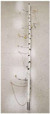
Sample pipe with heat wrap and insulation
