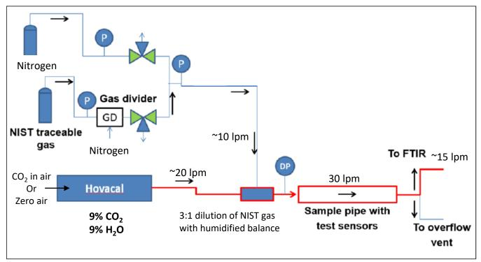
FIGURE 1. SCHEMATIC OF TEST SETUP FOR CALIBRATING SENSORS
