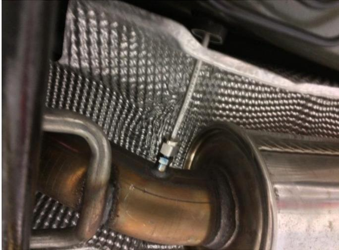
Fast [NO] sampling point: 40mm before silencer/muffler
