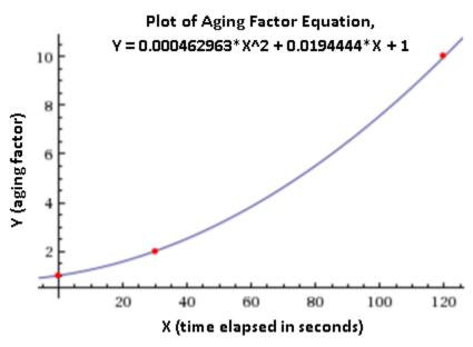
Fig. 11: Plot of Quadratic Aging Factor Equation
