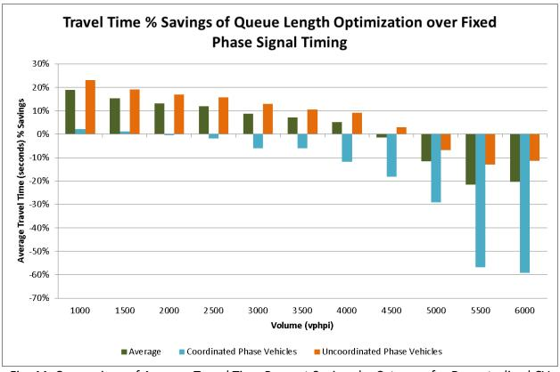
Fig. 44: Comparison of Average Travel Time Percent Savings by Category for Decentralized CV Queue Length Signal Optimization over Coordinated Fixed Phase Signal Timing on a 3-intersection Corridor
