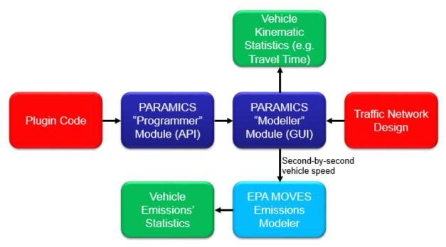
Fig. 12: Microscopic Traffic Simulation System Diagram
