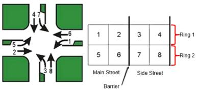
Fig. 5: Signal Phase Diagram & Dual-Ring Controller, adapted from [14]
