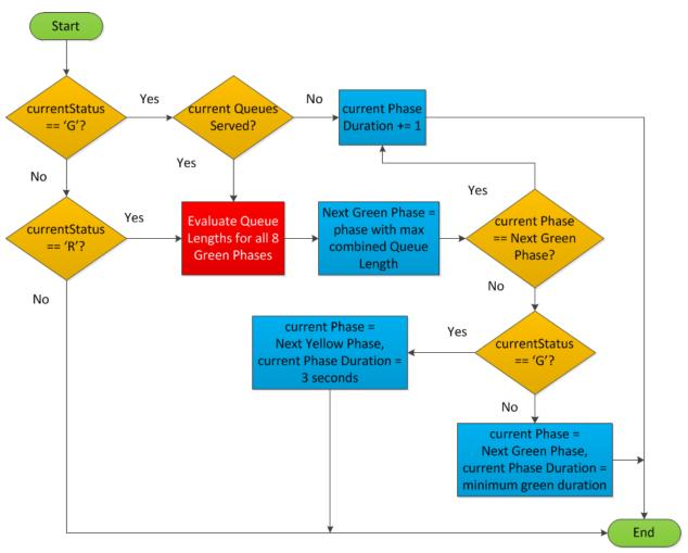
Fig. 10: CV MAS Level 2 Diagram: Queue Length Signal Optimizer
