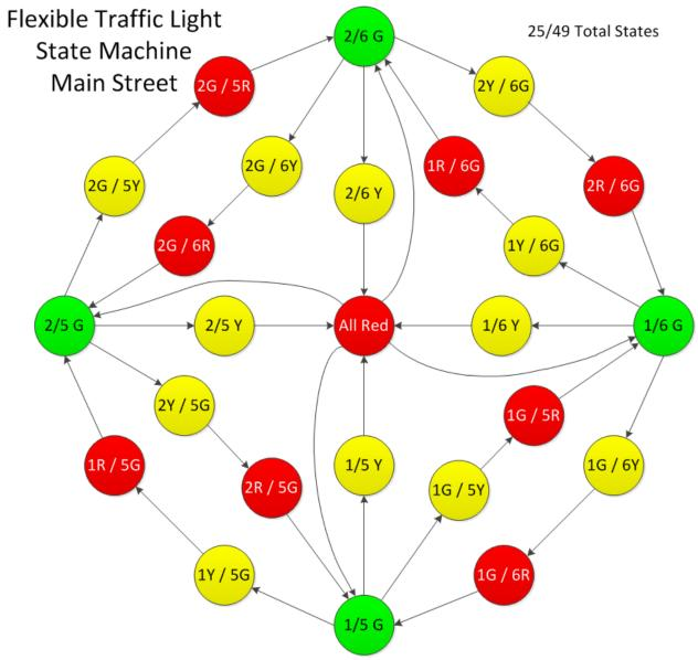
Fig. 8: Main street portion of Flexible Dual-Ring Controller, Finite State Machine Representation
