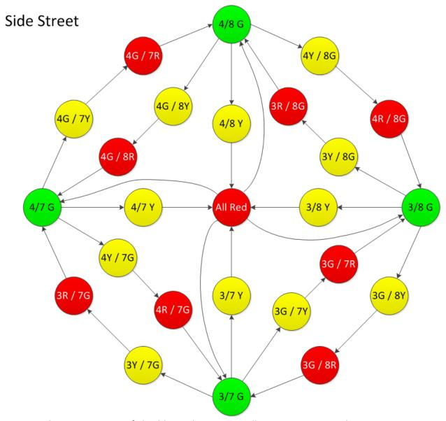
Fig. 9: Side street portion of Flexible Dual-Ring Controller, Finite State Machine Representation
