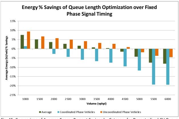
Fig. 45: Comparison of Average Energy Percent Savings by Category for Decentralized CV Queue Length Signal Optimization over Coordinated Fixed Phase Signal Timing on a 3-intersection Corridor
