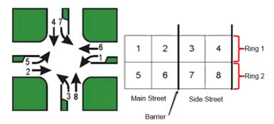
Fig. 1: NEMA Dual-Ring Phasing Diagram, adapted from [14]
