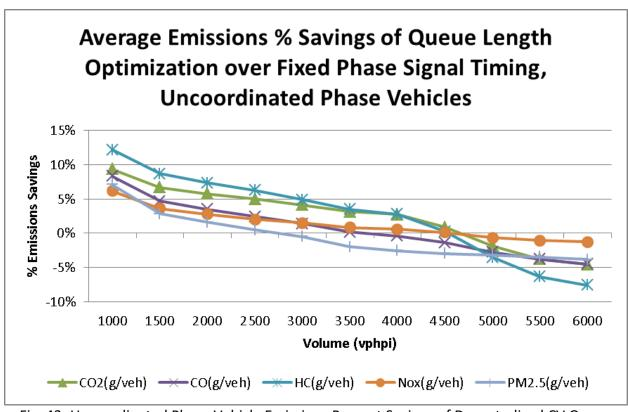
Fig. 43: Uncoordinated Phase Vehicle Emissions Percent Savings of Decentralized CV Queue Length Signal Optimization over Coordinated Fixed Phase Signal Timing on a 3-intersection Corridor
