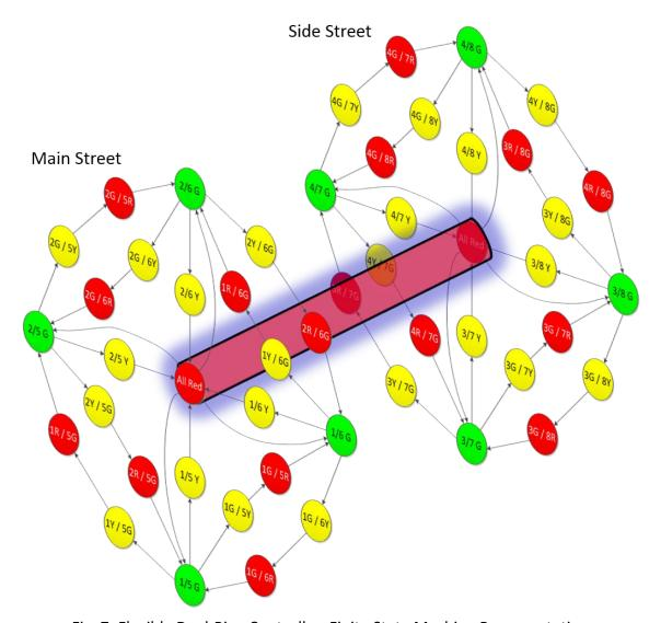
Fig. 7: Flexible Dual-Ring Controller, Finite State Machine Representation
