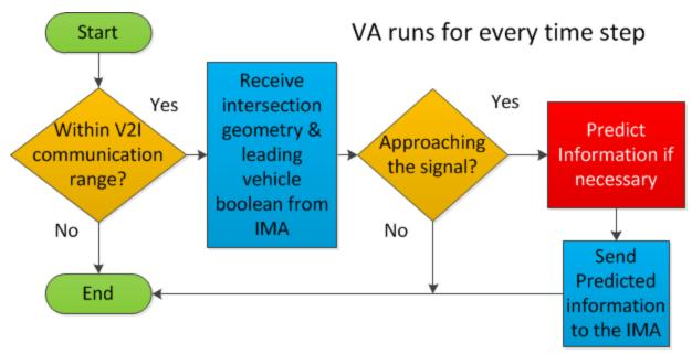
Fig. 4: CV MAS Level 1 Diagram: Vehicle Agent Flow Chart
