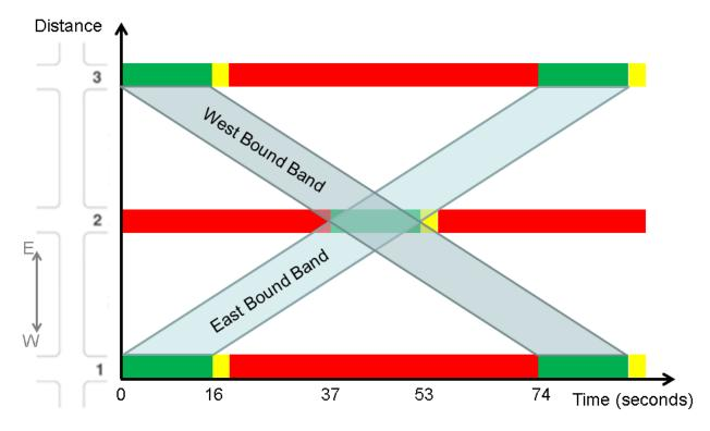
Fig. 28: Time-Space Diagram showing Coordinated Fixed Phase Signal Timing Plan for PARAMICS Network (see previous Fig.)
