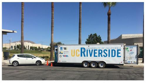
Shown in Picture: Electric Vehicle supplying power to the storage bank (inside trailer) which is connected to the building microgrid
