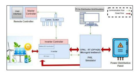
Power hardware-in-the-loop simulation of cyber-physical systems
