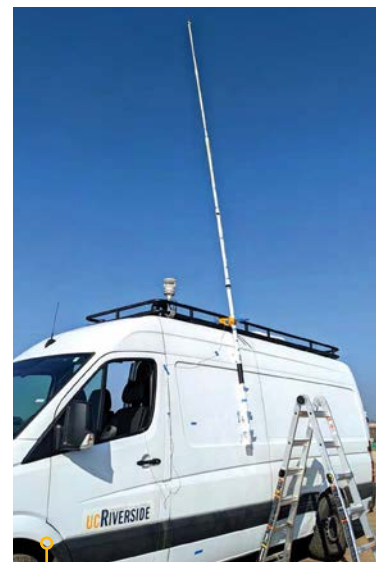
Mobile lab set up with an 8 meter mast for sampling around the dairy digester-lagoon complex.
