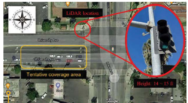
Riverside's Innovation Corridor with UCR's smart intersection testbed to evaluate connected vehicle scenarios.
