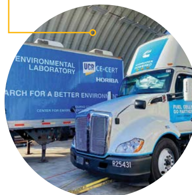
Testing a Fuel Cell Vehicle on the CE-CERT Heavy Duty Chassis Dynamometer
