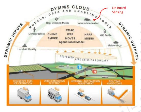
• The Dynamic Mobility Management System will collect data from vehicles, the transportation system, and the atmosphere and use these inputs to implement real-time decisions on vehicle behavior and energy management.
