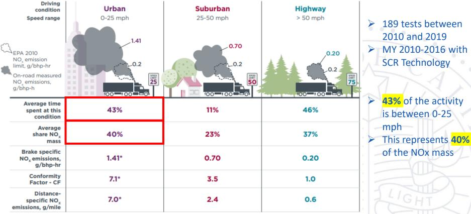
\* Brake and distance specific NOx emissions for Urban bin do not include Idle operation, only 1-25 mph operation is included
