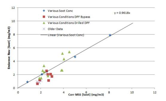
In 2013, GM tested the EmiSense electrostatic sensor and found that it had good correlation with matching the soot concentration reported by the MSS at a wide range of different supplied soot rates.
