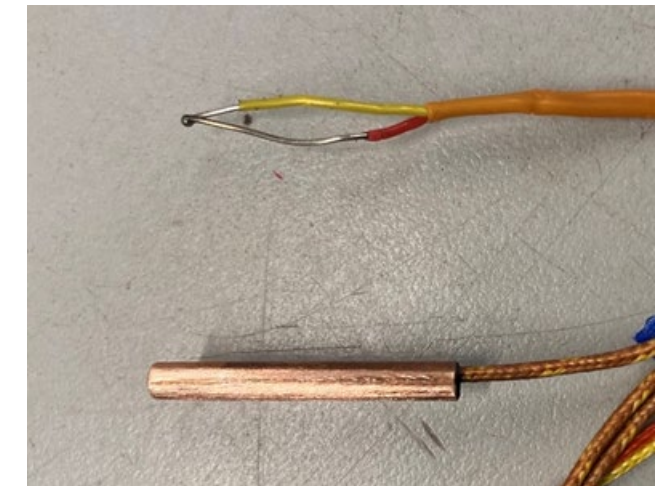
Probe tips: brake test probe (bottom) used in the study and exposed tip (top).
