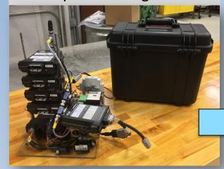
Design Includes: Control Modules, DAQ, Data Logger, Battery (8 hours) and Barometric Pressure
