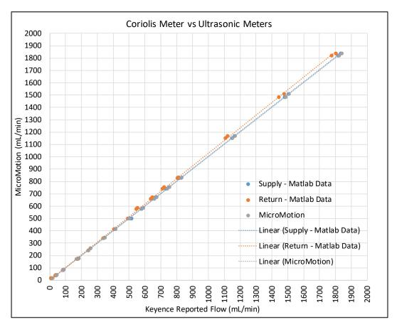
Typical range: 25 to 1,700 mL/min (+/- 5% above 40 mL/min)
