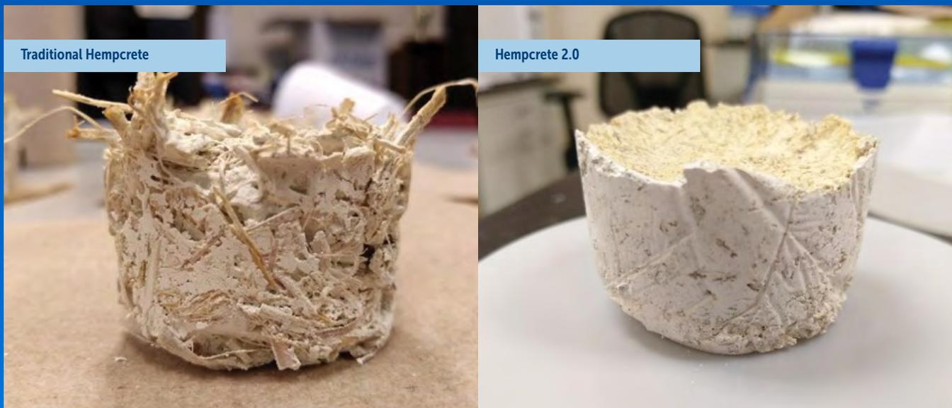
Hempcrete made from raw decorticated hemp hurd (left) and CELF pulped hemp stalk (right). Our team recently demonstrated a stronger and more insulating Hempcrete 2.0 than traditional hempcrete. The samples pictured were produced using identical 1.1:3 (biomass:binder:water) ratios in formulation. Funding from US EPA.
