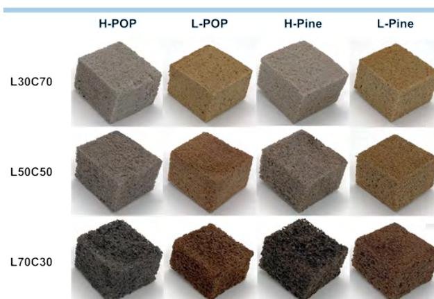
Lignin-based non-isocyanate polyurethane (lignin-NIPU) insulating foams were successfully synthesized in a room temperature solvent-free system from pine wood and poplar (POP) wood lignin, incorporating 30-70% CELF lignin. These foams seek to replace conventional polyurethane insulation in homes and commercial buildings. Funding from US ARPA-e.
