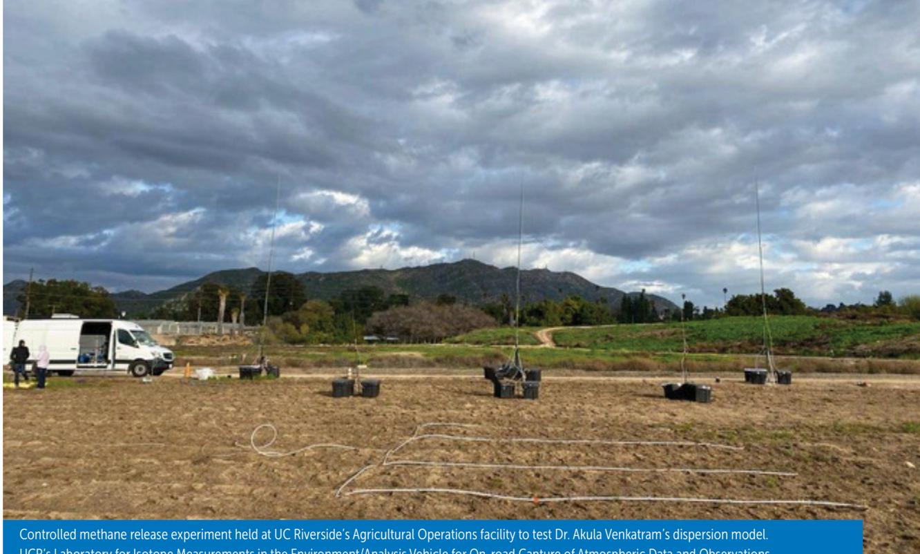
Controlled methane release experiment held at UC Riverside's Agricultural Operations facility to test Dr. Akula Venkatram's dispersion model. UCR's Laboratory for Isotope Measurements in the Environment/Analysis Vehicle for On-road Capture of Atmospheric Data and Observations (LIME/AVOCADO) shown in the background (photo credit: Dr. Javier Gonzalez Rocha)
