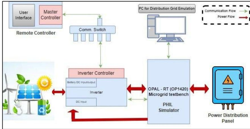
Power hardware-in-the-loop simulation of cyber-physical systems
