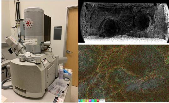
**Scanning Electron Microscopy / Energy Dispersive X-ray spectroscopy (SEM/EDS)**
