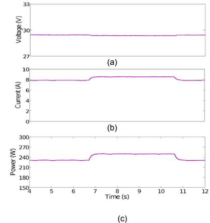
Hardware test- DG#2 performance during load change: a) Voltage at dc link, b) dc-dc converter inductor current, and c) DG output power
