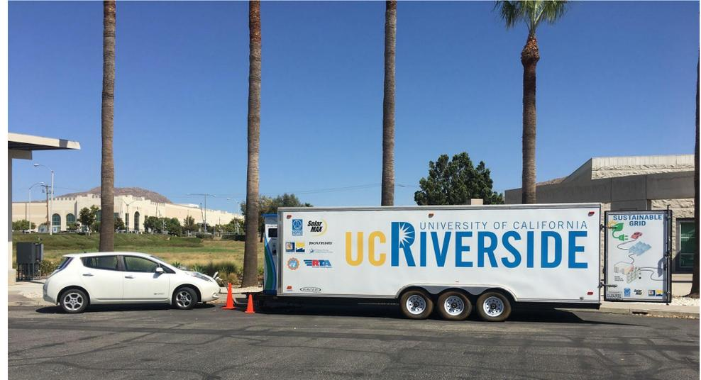
*Shown in Picture: Electric Vehicle supplying power to the storage bank (inside trailer) which is connected to the building microgrid*
