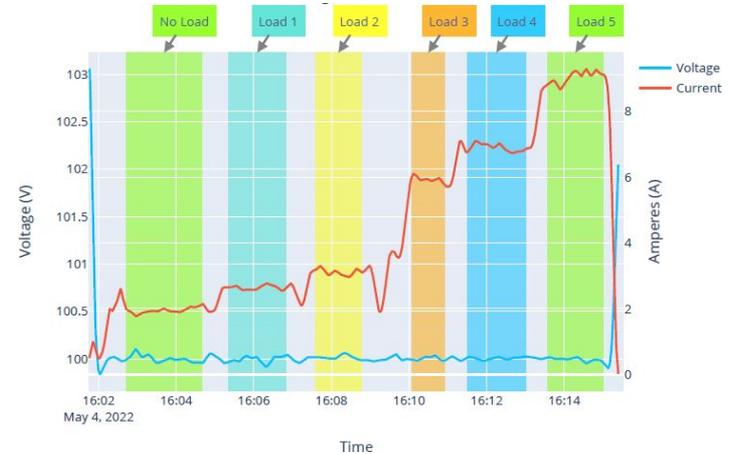
Input Voltage and Current at 1,000 RPM
