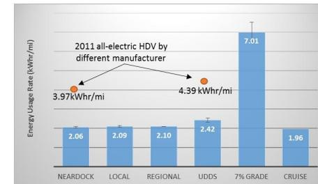
***Electric Vehicle Drive Cycle Testing***
