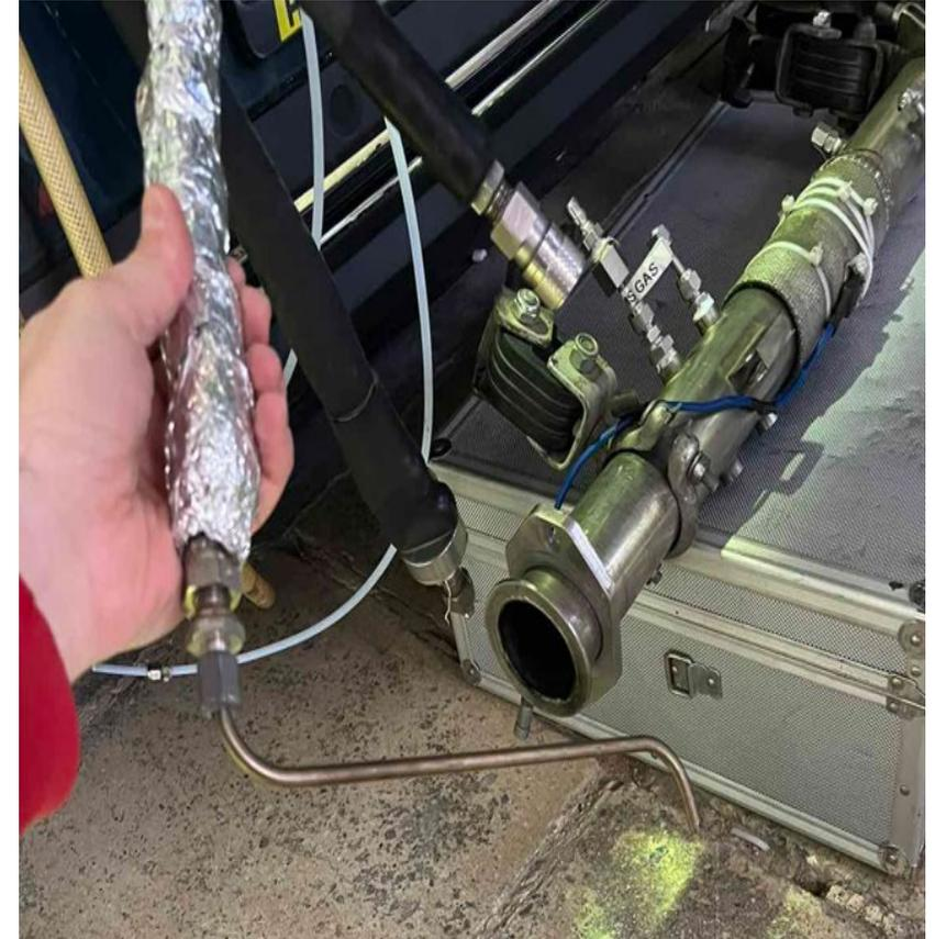
*Exhaust pipe and heated line*
