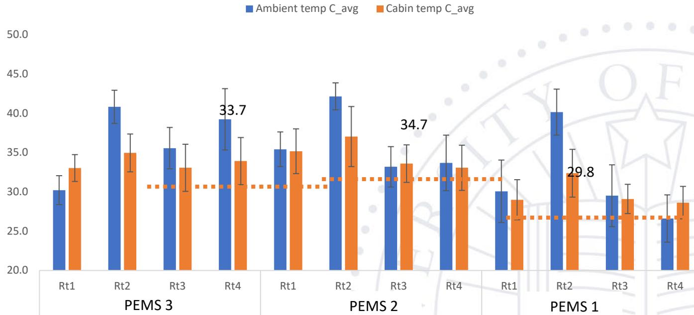
➤ **PEMS 1 was subjected to a slightly lower cabin temperature (5 deg C lower) compared to PEMS 2 and 3**
