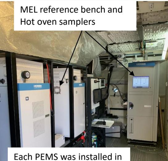
Each PEMS was installed in the sleeper area of the Class 8 truck
