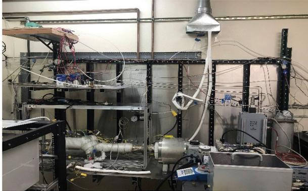
High flow bench to simulate exhaust conditions while calibrating and comparing with an FTIR and PM (miniCAST)
