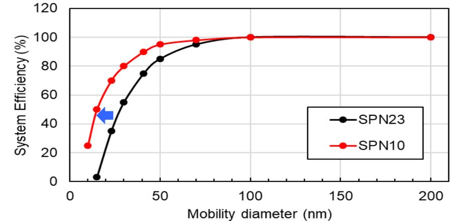
Expansion of system detection lower limit (23nm → 10nm)
