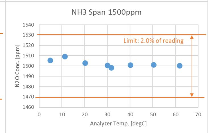
\*X-axis of graph: Temperature inside analyzer
