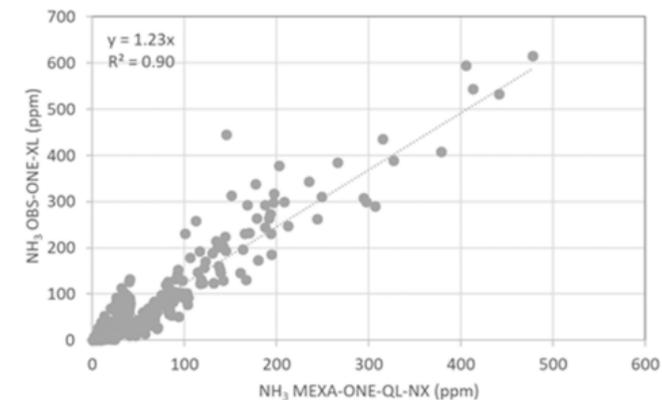
On the road, the correlation of the N<sub>2</sub>O concentrations measured by the two on-board systems, OBS-ONE-XL and PEMS-LAB, was good, with an R<sup>2</sup> = 0.95 obtained. In the case of the NH<sub>3</sub> emissions, the OBS-ONE-XL showed a more accurate performance, with sharper, better defined peaks, and less tailing effects related to NH<sub>3</sub> adsorption on the setup obtained
