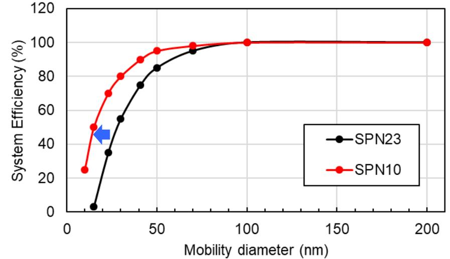
Expansion of system detection lower limit (23nm → 10nm)
