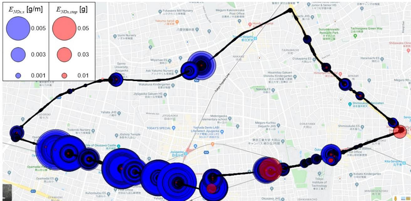
Distance-based  $NO_x$  mass emissions for diesel passenger vehicle
