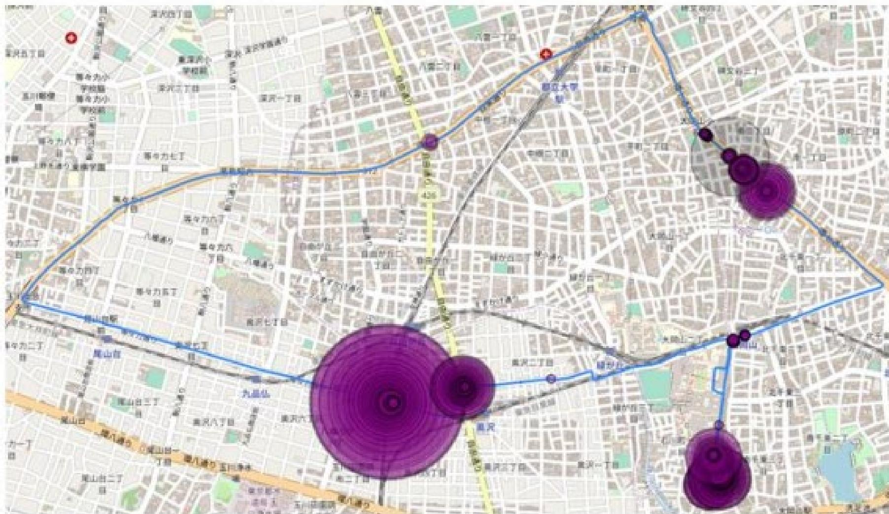
1. PM emission increased during rapid acceleration and even more so when vehicle reaccelerates after deceleration.
