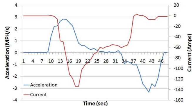
The graph above shows the relationship between the acceleration and the current drawn from the vehicle. The reason why the current is negative is because it current coming out of the batteries. As acceleration increases the current drawn also increases. As acceleration decreases the current drawn also decreases.
