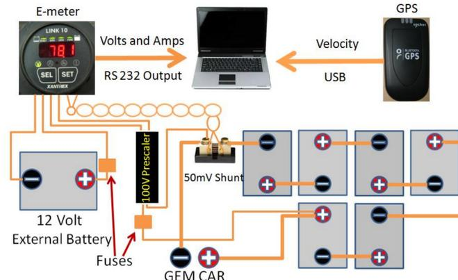
The block diagram above shows how the e-meter was The laptop recorded all the data from the e-meter and GPS using matlab.
