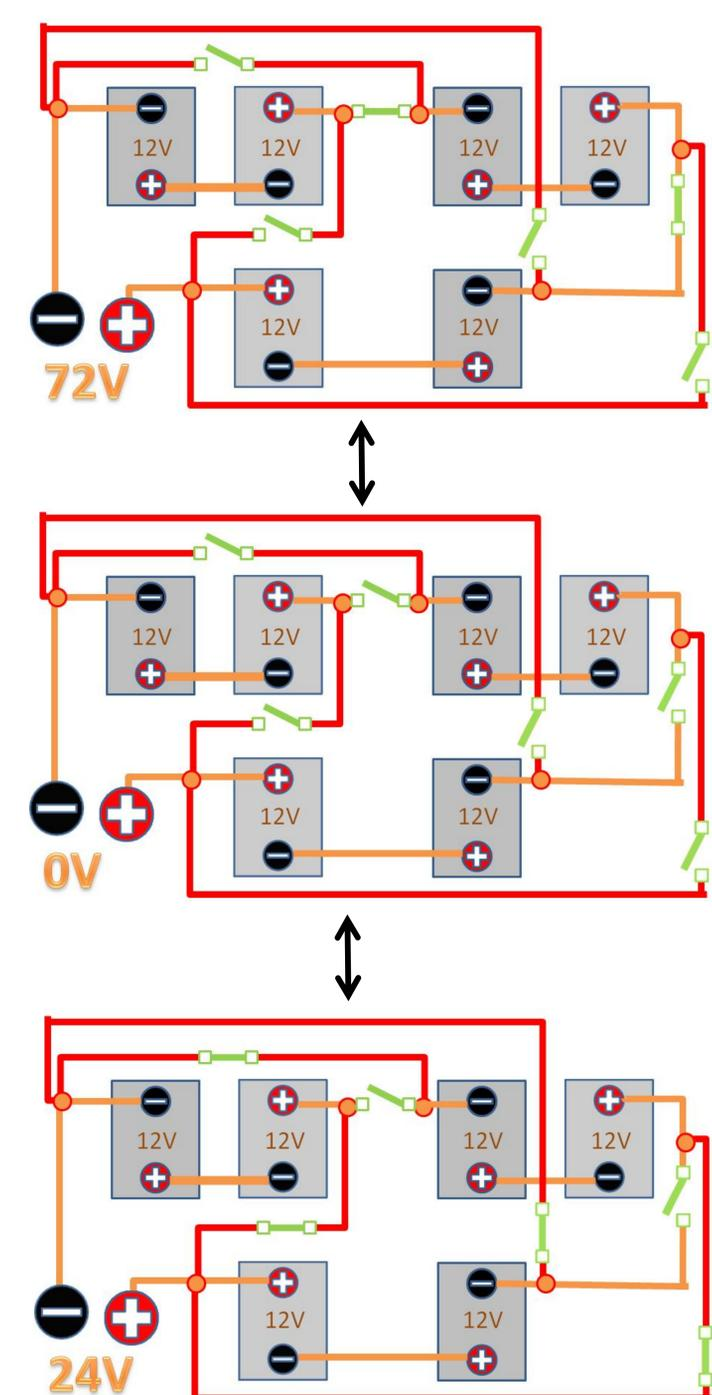
The diagrams above shows the transition of the circuit conversion from 72V to 24V using solenoids. The voltage drop is necessary because the solar panels do not produce enough voltage to charge at 72V, therefore the batteries will charge at 24V.
