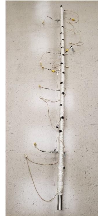
**Sample pipe with heat wrap and insulation**
