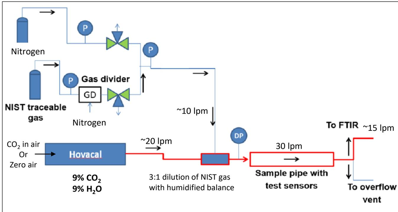
FIGURE 1. SCHEMATIC OF TEST SETUP FOR CALIBRATING SENSORS
