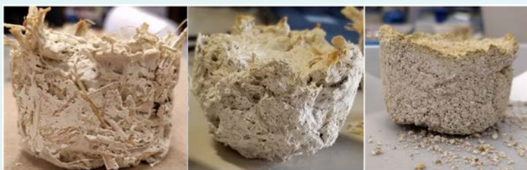
Traditional hempcrete made with untreated hemp hurds (left); experimental hempcrete made CELF-treated hemp fibers (center); and agitated CELF-treated fibers (right)
