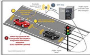
DSRC Enabled Traffic Lights
