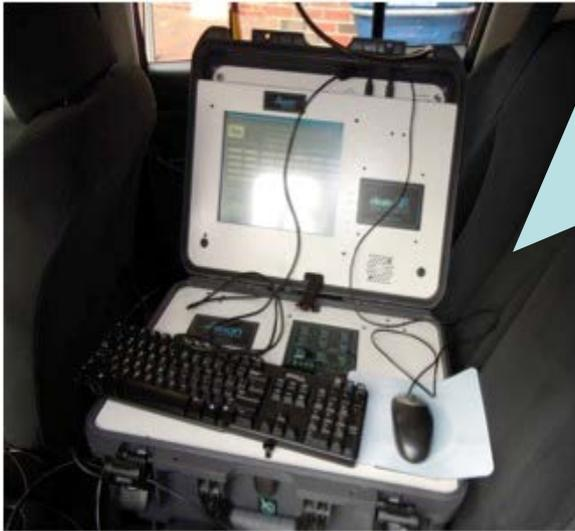
Portable Emissions Measurement System (PEMS):
