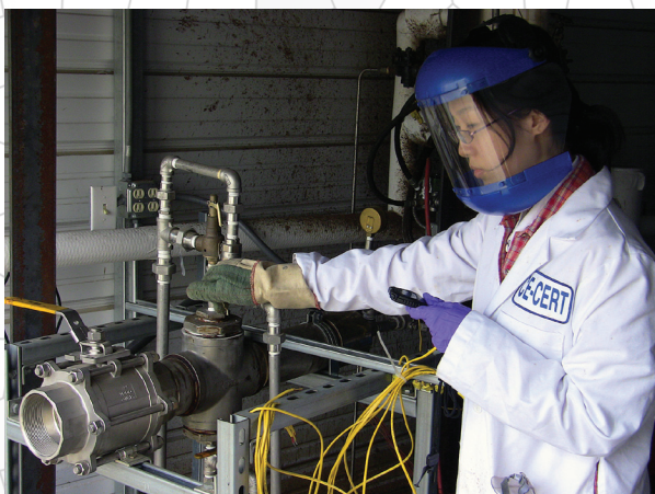
Lignocellulose pretreatment, particularly research on continuous feed fermentation, requires a custom-designed, high-yield steam gun which can deliver 60 percent solid load processing at high pressure and 180-260 degrees Celsius.
