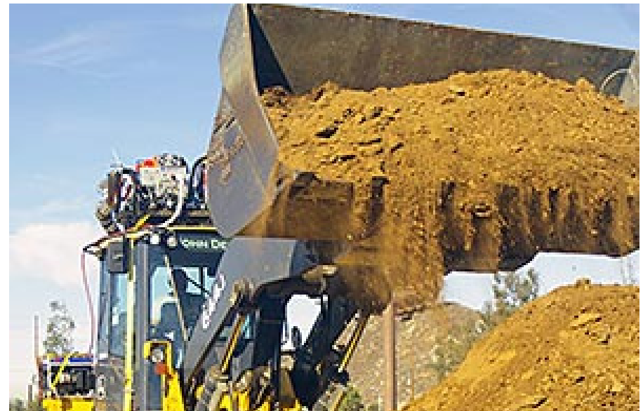
PEMS equipment, seen on the roof of this tractor, captures the behavior of hybrid equipment on a second by second basis during in-use operations at construction sites.
