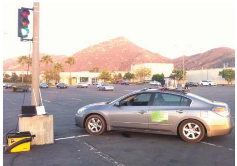
*The combination of instruments mounted on the vehicle and the pole-mounted equipment made up the test bed for vehicle positioning research for the Federal Highway Administration.*
