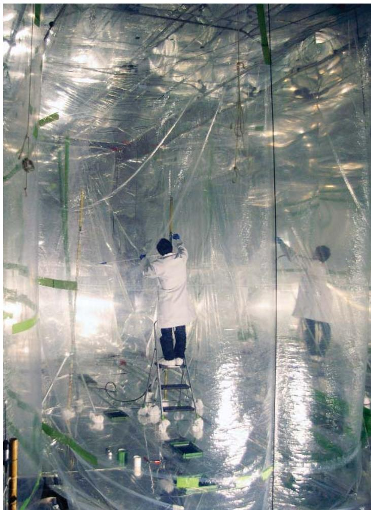
*Shunsuke Nakao works through the painstaking process of ensuring the bag is sealed tight before an experiment.*
