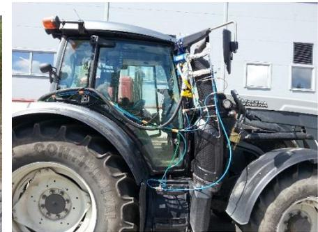
**Platform for different exhaust emission measurements**
