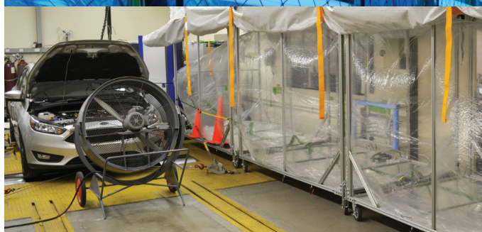
Studying secondary aerosol formation from a variety of fuels in the Portable Chamber.
