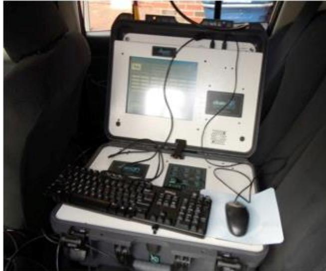
Portable Emissions Measurement System (PEMS)
