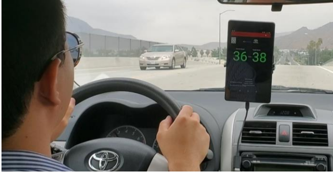
Fig. 8. A driver is tracking ASA on HMI in a real passenger vehicle.
