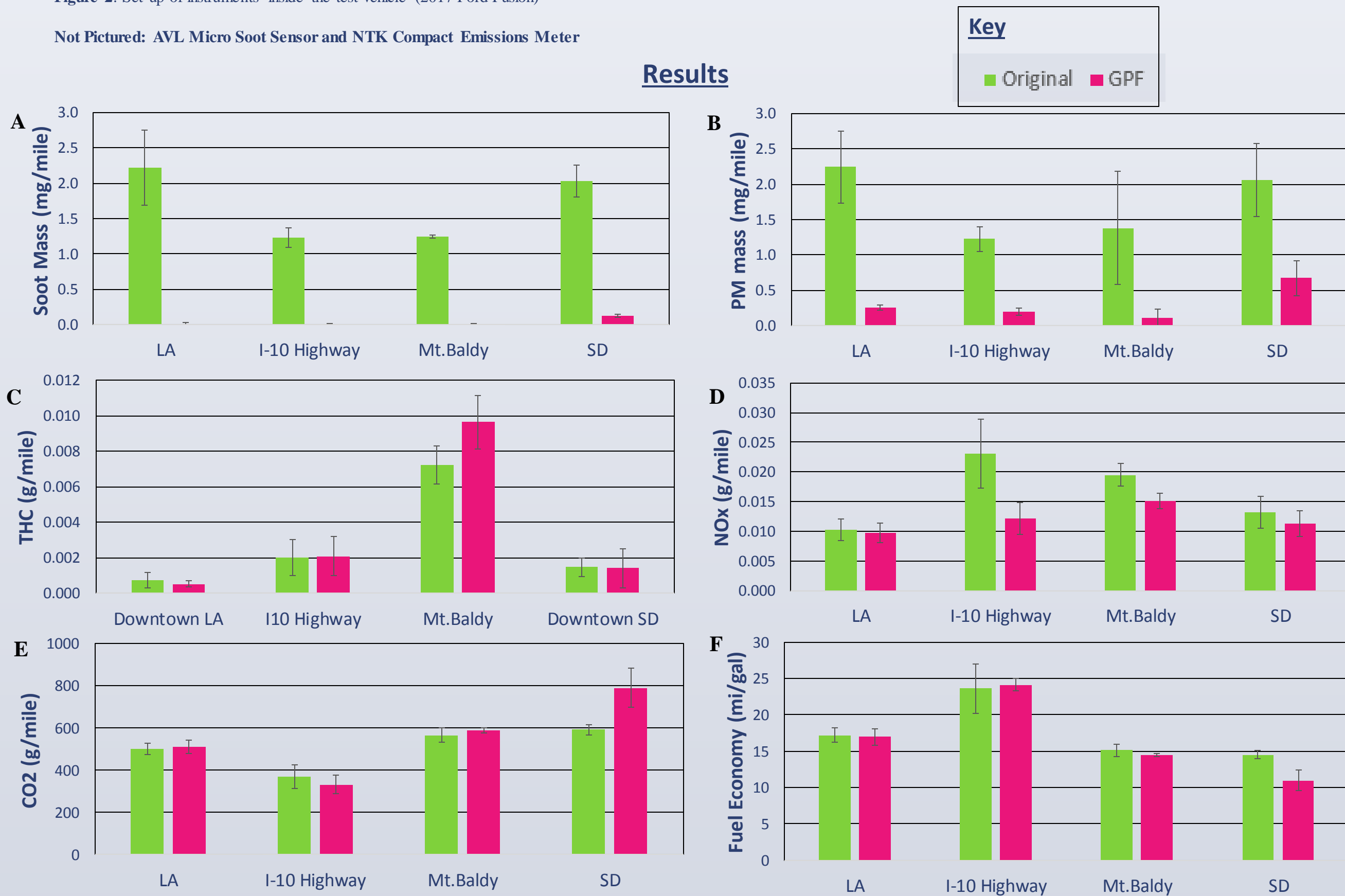
Figure 3: Comparison of GPF and non-GPF after treatment for the 4 routes based on soot mass (A), PM (b), THC (c), NOx (d), and CO2 (e) emitted per mile as well as fuel consumption (f).
