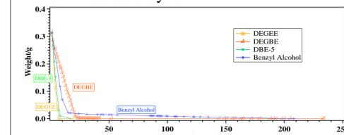
Fig 6. LVP-VOCs weight loss in evaporation chamber
