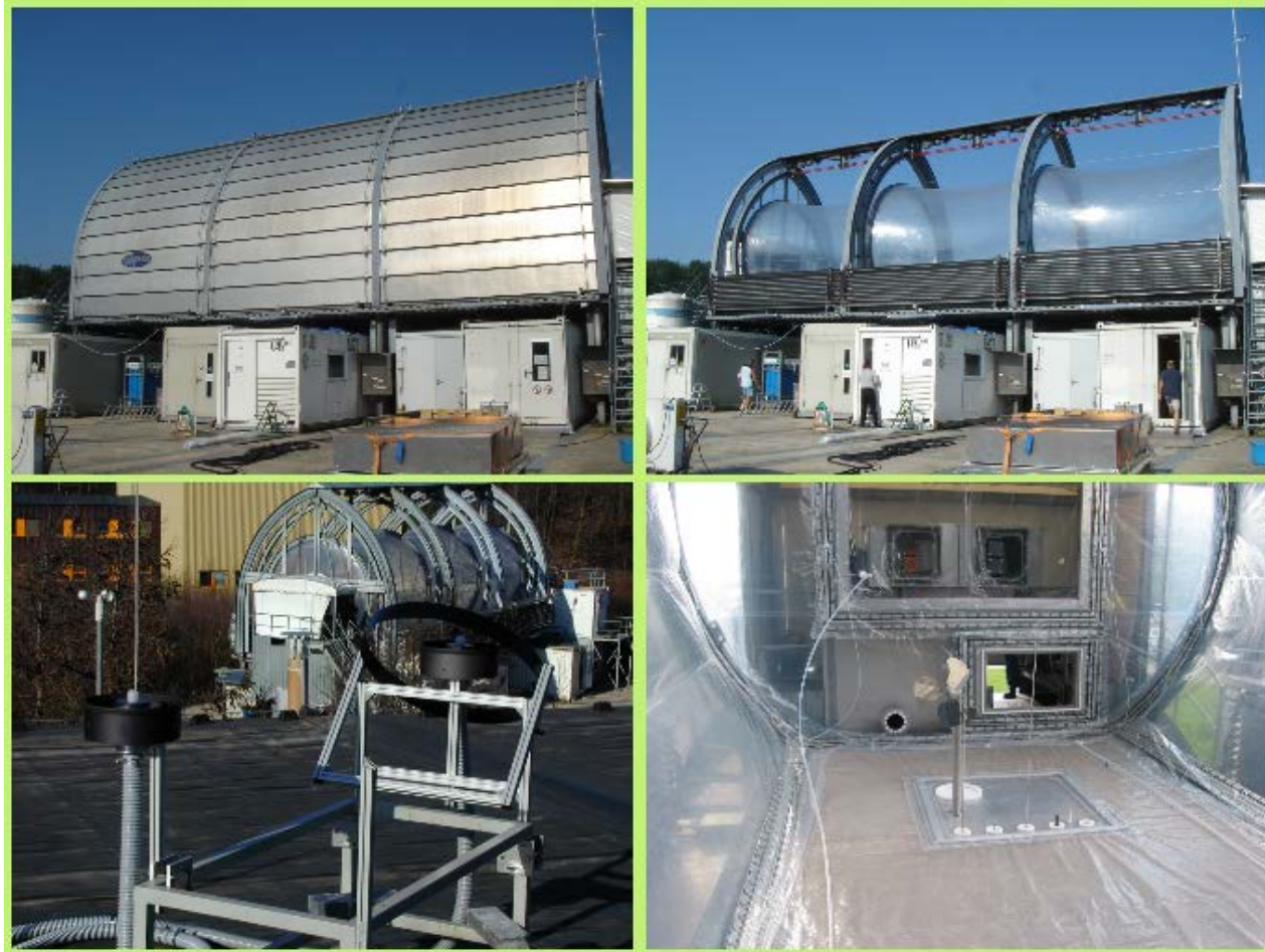
Simulation of Atmospheric PHotochemistry In a large Reaction (SAPHIR) chamber in Jülich, Germany ( http://www.eurochamp.org/chambers/saphir/ ): 270 m 3
