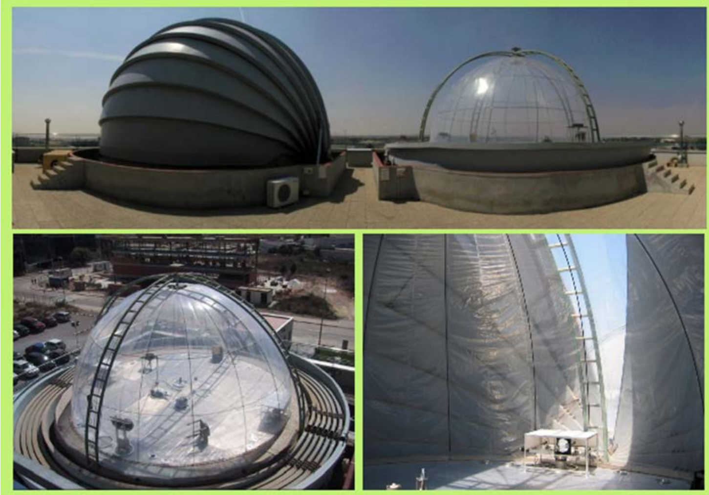
EUPHORE (European PHOtoreactor) chamber in Valencia, Spain ( http://www.eurochamp.org/chambers/euphore ): volume = 200m 3 each.
