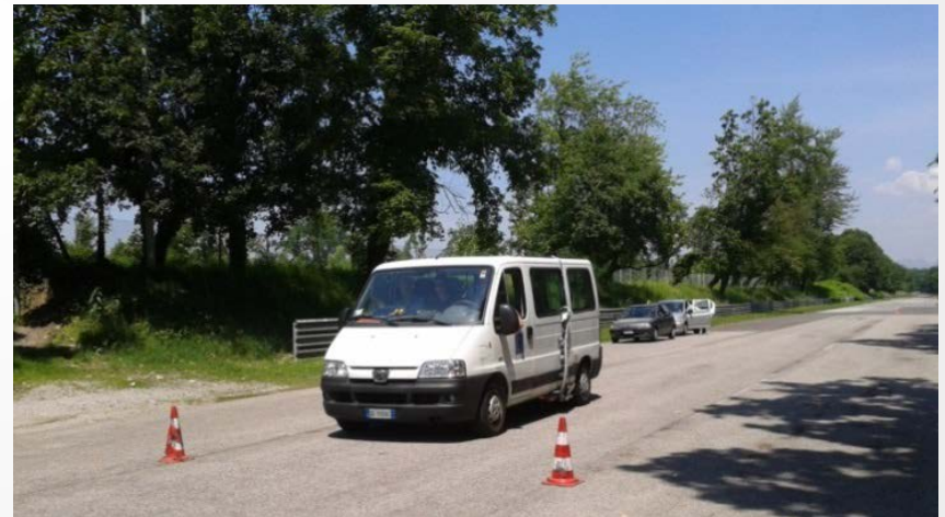
The van equipped with PEMS on the old part of the Monza F1 race track (Italy)
