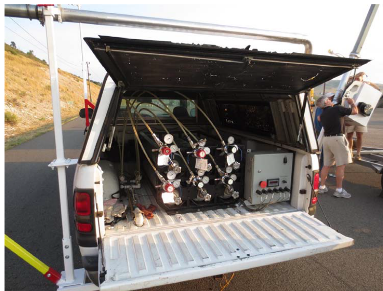
Figure 2. RSD Audit Truck with Engine Exhaust 10-foot Side Extension
