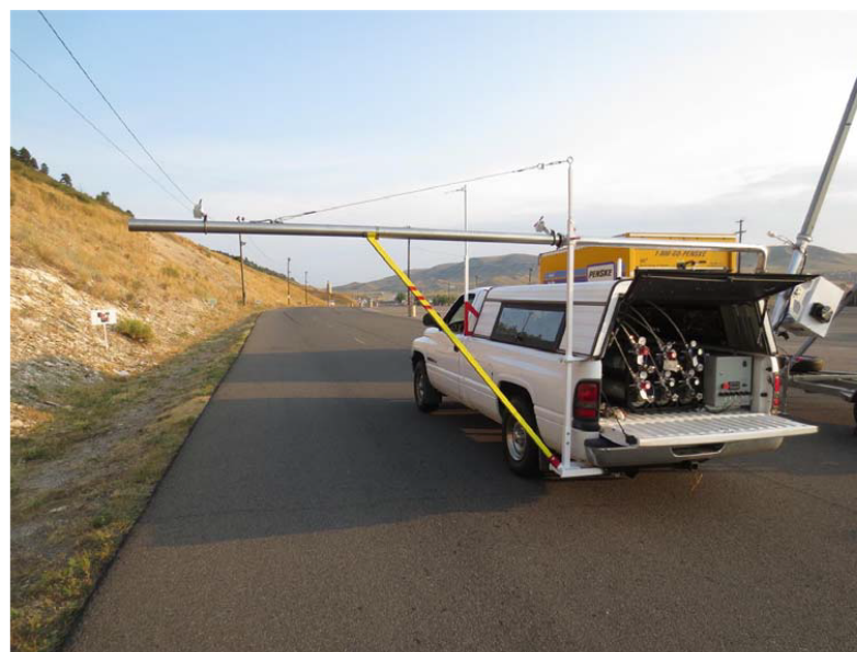
Figure 2. RSD Audit Truck with Engine Exhaust 10-foot Side Extension
