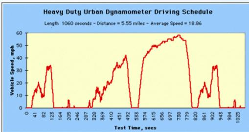
PEMS testing – Source cycle      Virtual Chassis Dyno Lab
