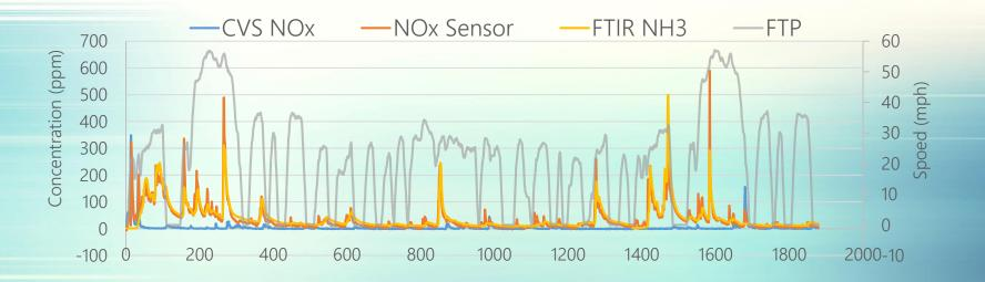
FTIR readings in the dyno identify NH<sub>3</sub> emissions previously reported by the sensor as NO<sub>X</sub> emissions during on-road screening.
