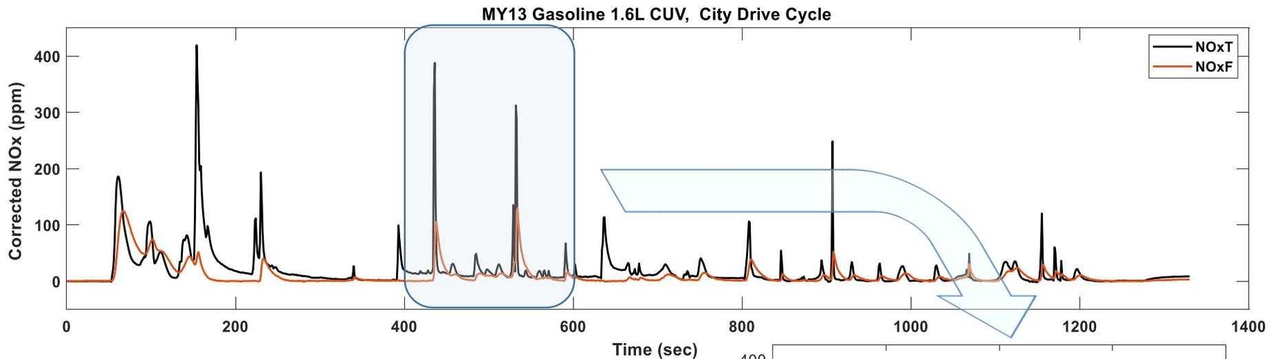
NOxF Signal Must be Advanced 2 sec to align with NOxT and Mass Flow
