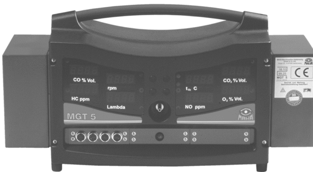
Figure C-1 Emissions Analyzers for Chassis Dynamometer Measurements
