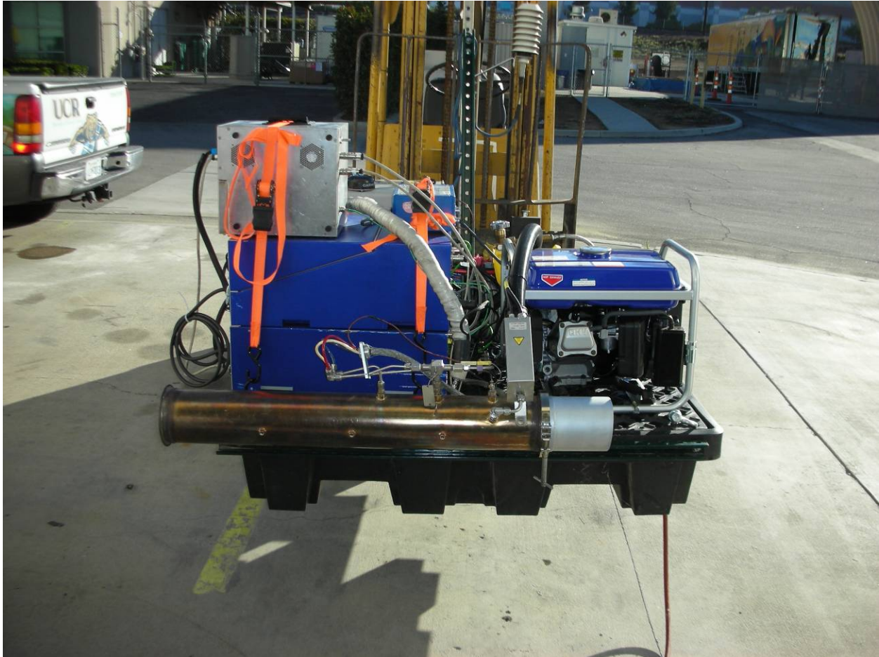
Figure B-6: Emission analyzers, generator, and flow meter on a 4' by 4' Plastic Pallet
