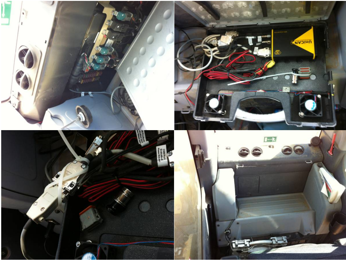
Figure 4-2: UniCAN Pro Installed in a Wheel Loader
