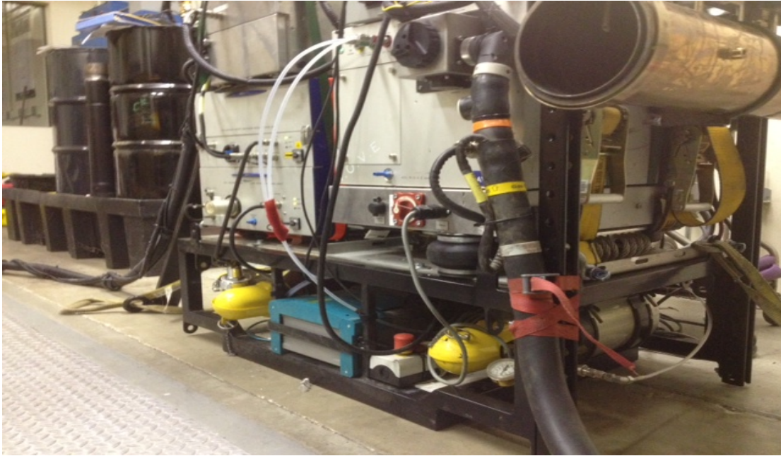
Figure B-7: Platform with emission measurement equipment used for the last seventeen tests
