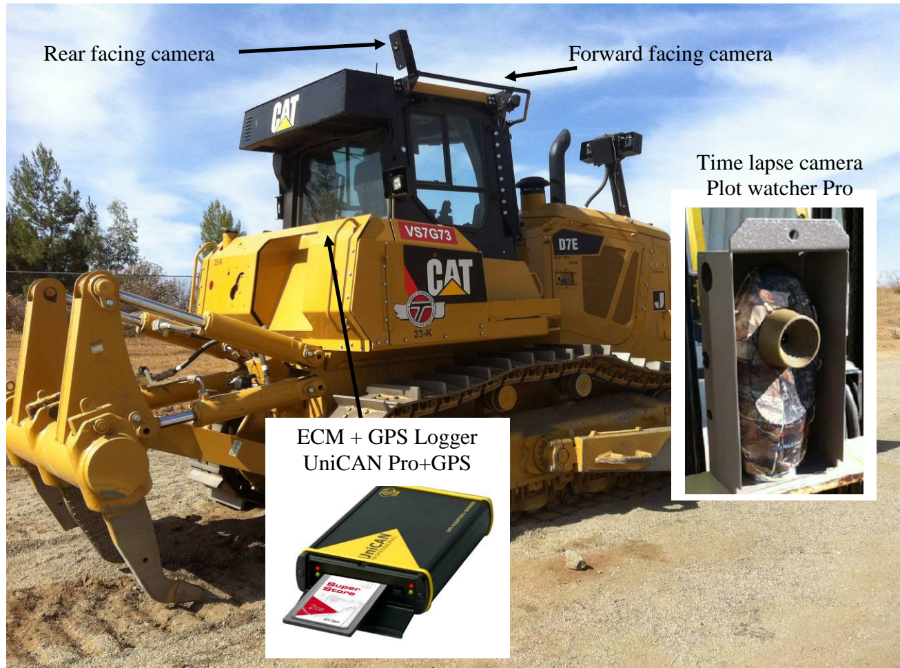
Figure B-14: Activity measurement tools ECM, GPS, and time lapse video on the D7E
