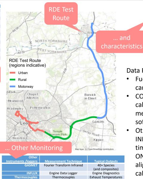
Value 97.2 km **Urban Distance Share** 31.5 - 37.7 %**Rural Distance Share** 29 - 35.6 % **Motorway Distance Share** 29.6 - 35.2 % **Urban Speed Range**  $0 - 60 \, \text{km/h}$ **Rural Speed Range**  $60 - 90 \, \text{km/h}$ **Motorway Speed Range** >90 km/h **Average Test Duration** 1 hr 54 min  $24 - 103 \, \text{m}$ **Cumulative Elevation Gain** 563 m/100km
