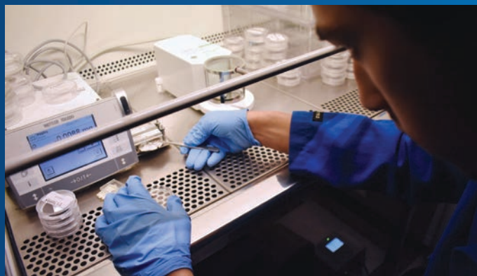
GRADUATE STUDENT ANTHONY GERIGK WEIGHS THE FINAL MASS OF EMISSIONS ON A TEFLON FILTER
