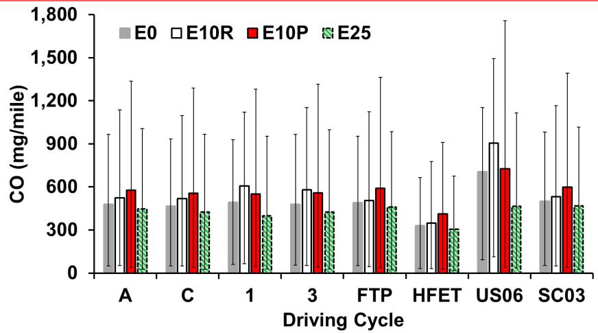
Note: Error bars are 95% confidence intervals (CIs) based on mean cycle-average CO emission rates for 5 vehicles for each driving cycle, and are estimated using bootstrap resampling for negative CIs.
