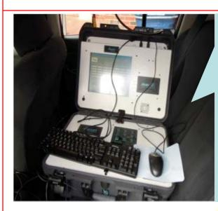
Portable Emissions Measurement System (PEMS): Carbon Dioxide (CO<sub>2</sub>), CO, and Hydrocarbons (HC)- NDIR Nitric Oxide (NO) – electrochemical PM – laser light scattering
