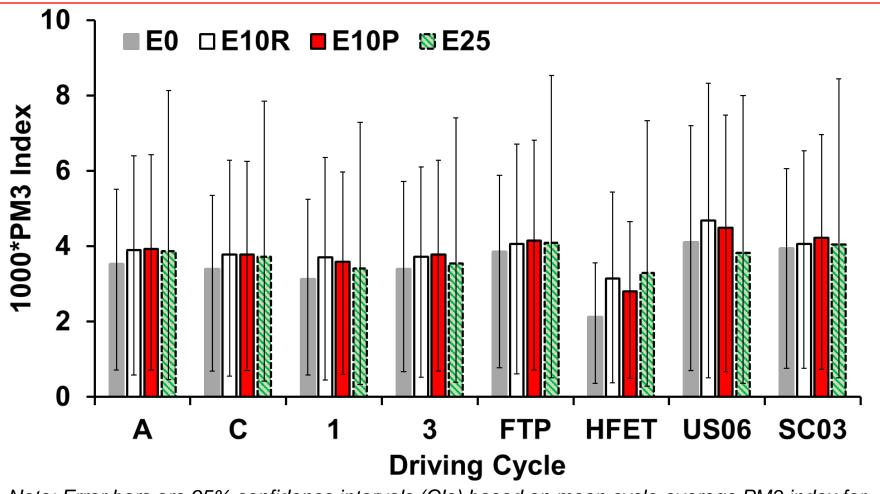
Note: Error bars are 95% confidence intervals (CIs) based on mean cycle-average PM3 index for 5 vehicles for each driving cycle, and are estimated using bootstrap resampling for negative CIs.
