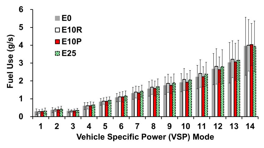
Note: Error bars are 95% confidence intervals based on mean fuel use rates for 5 vehicles for each VSP mode.
