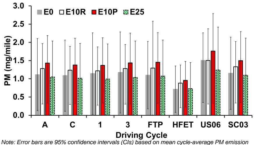
Note: Error bars are 95% confidence intervals (CIs) based on mean cycle-average PM emission rates for 5 vehicles for each driving cycle, and are estimated using bootstrap resampling for negative CIs.
