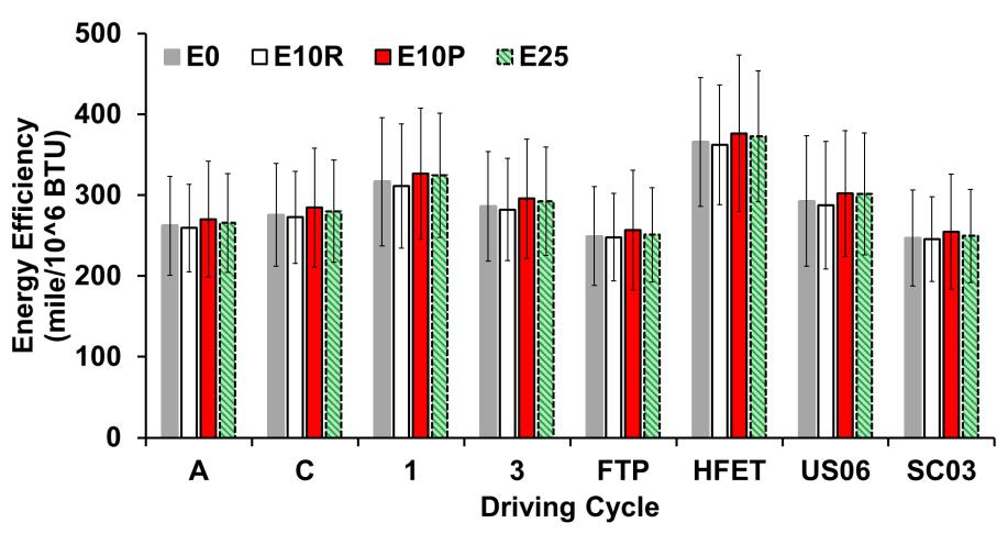
Note: Error bars are 95% confidence intervals based on mean cycle-average energy efficiency for 5 vehicles for each driving cycle.
