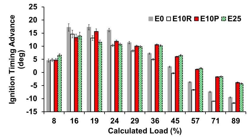
Note: Error bars are 95% confidence intervals based on mean ignition timing advance for each engine calculated load bin for the Cruze.
