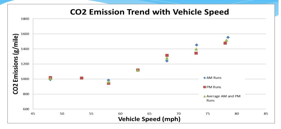
• Sweet spot w.r.t. fuel efficiency around 58 mph (engine speed ~1250 rpm)
