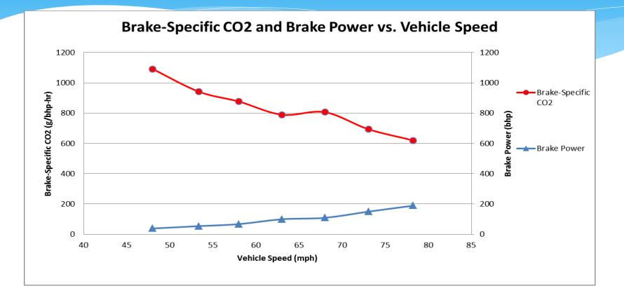
Brake specific fuel efficiency improved at higher speed; however, power demand increased at higher speed.
