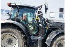
Platform for different exhaust emission measurements
