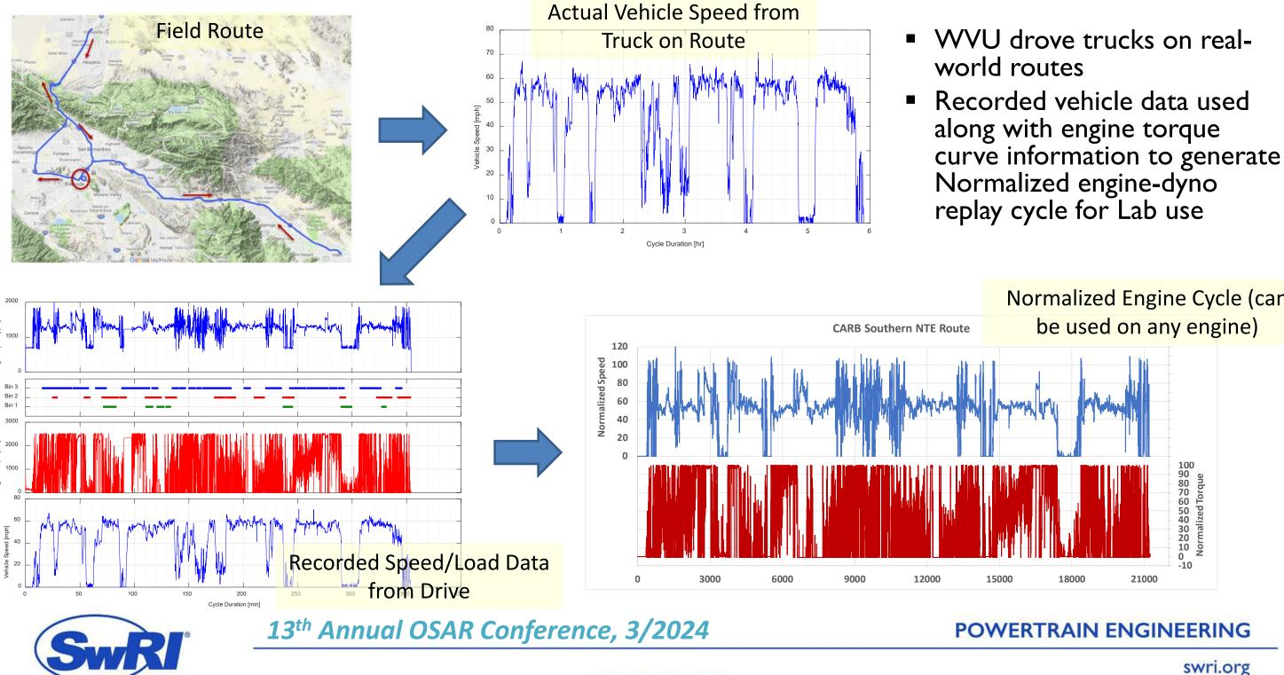
Normalized Engine Cycle (can be used on any engine)
