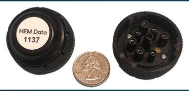
Note: Streamer uses WiFi and is designed for HD OBD SAE J1939 protocol but can use converter cable to evaluate OBD-II SAE J1979 protocol
