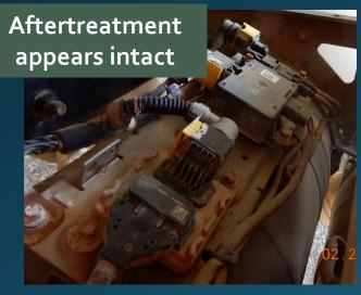
Veh 27 — Discrete Delete (only detected through OBD Data)
