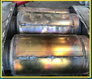
SCR canisters welded shut
